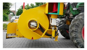
Easy to empty the compressor when you reverse the direction of rotation of the auger.
